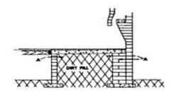
Figure 5—Dirt Filled Step
